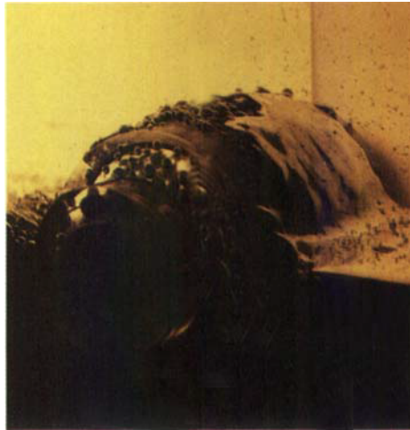
FIGURE 21. A combination of emulsion and sheet coating of 1% polyacrylamide/water (blue) in castor oil (yellow).
